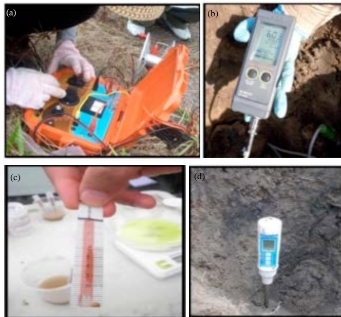
Fig. 2(a-d): In-situ parameter measurement, (a) Soil resistivity, (b) pH, (c) Chloride and (d) Moisture content
