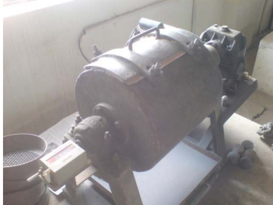
Fig. 1: Ball mill used for grinding ceramic tiles
