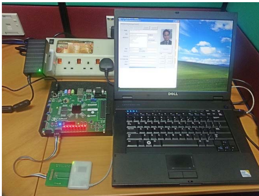
Fig. 9: Real-time testing of the ARM-based FPGA prototype smart card
