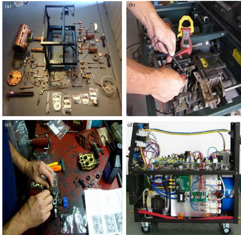
Fig. 1 (a-d): Phases of the multi-server system, (a) Dissociation of the machine, (b) Repairing of machine (Electrical), (c) Repairing of machine (Mechanic) and (d) Installation of machine parts
