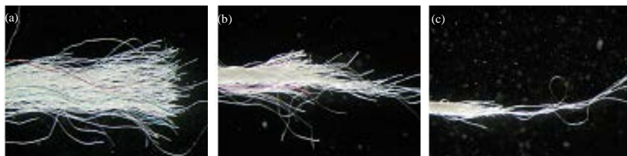
Fig. 2: Classification of broken ends structure: (a) sharp broken end (b) tapered broken end and (c) slipped broken end
