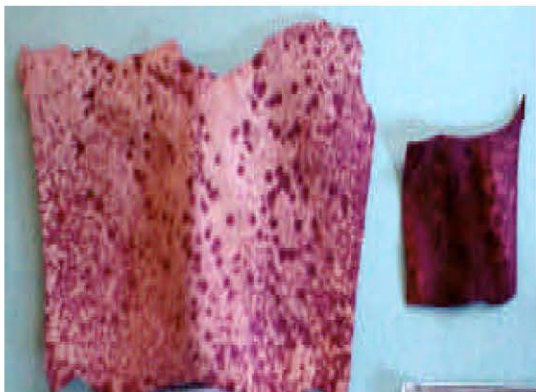
Fig. 3: Enhanced colonization and degradation of small sized NR-latex gloves (right) and large sized NR-latex gloves (left) by Nocardia sp. strain-MBR
