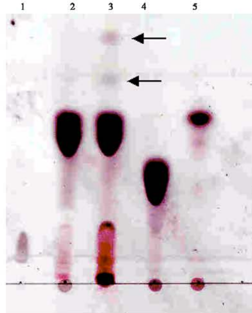
Fig. 4: TLC of the reaction products from crude and purified sucrose phosphorylase with sucrose. Glucose-1-phosphate standard (lane 1), crude enzyme reaction with sucrose (lane 2), purified enzyme reaction with sucrose (lane 3), sucrose standard (lane 4), fructose standard (lane 5) and arrows indicates the reaction by product
