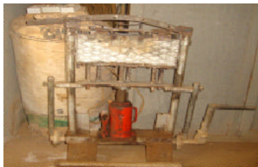
Fig. 2: The manual hydraulic briquetting machine
