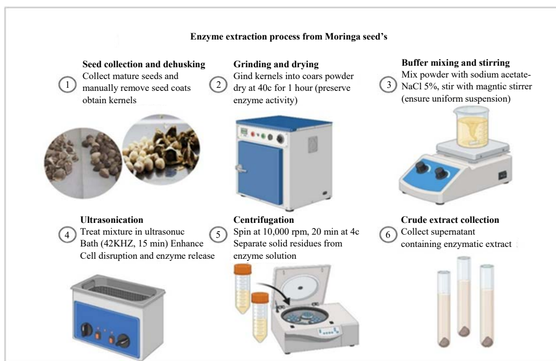
Fig. 1: Illustration of the crude extract preparation from Moringa seeds
