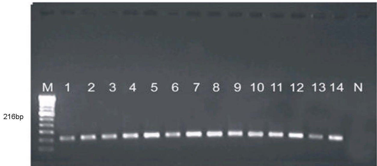
Fig. 2: Agarose gel electrophoresis of 216 bp nested PCR products generated from field isolates and reference strains using primer pair no. 2
