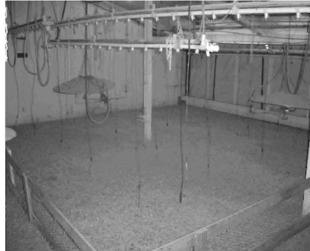
Fig. 2: Photograph of pen area. Thermocouples are suspended from the ceiling and spaced on 1 m intervals in a 5 x 5 grid.
