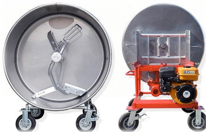
Fig. 1: Pictures of a flat-bottom vertical mixer with a capacity of 250 liter, 460 mm height and 900 mm diameter
