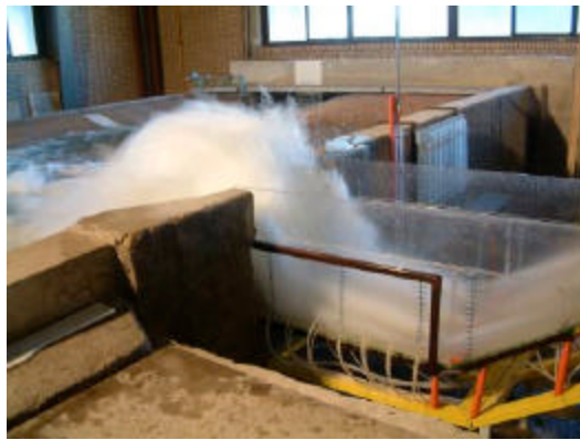
Fig. 11: Flow condition for 178 \text{ L sec}^{-1} discharge (parallel walls)
