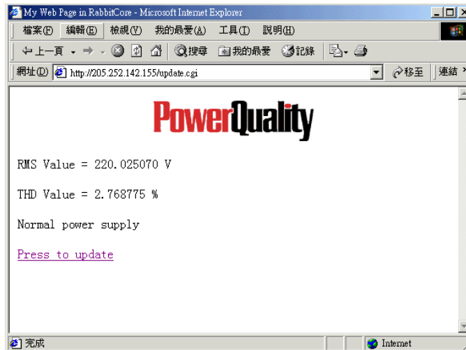
Fig. 5: The outlook of the power quality web page retrieved from the RCM2200 module
