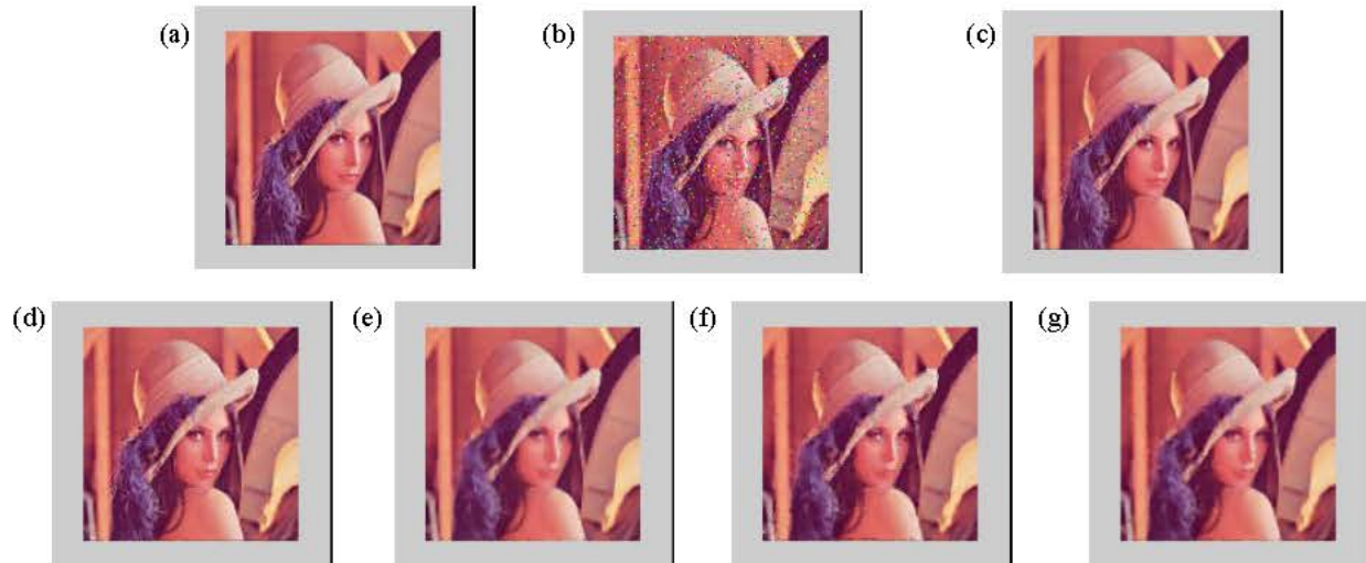
Fig. 1: Noise reduction effect of the proposed filter as compared with the adaptive filter [7] , VMF, BVDF and DDF: (a) color test image LENA, (b) image distorted by 5% impulsive noise, (c) the proposed filter, (d) the adaptive filter [7] , (e) VMF, (f) BVDF, (g) DDF
