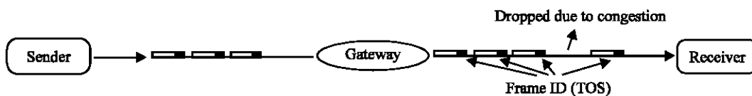
Fig. 2: Dropping packets due to congestion coherence using TOS field
