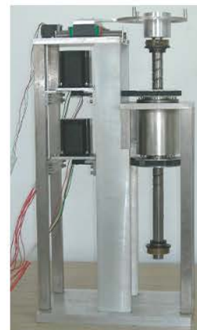
Fig. 1: The basic machine of wafer pre-aligner system (a) architecture and (b) Prototype
