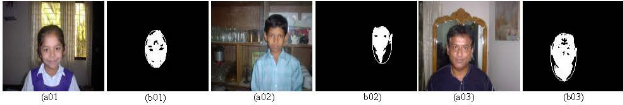
Fig. 4: Face detection for the persons at their work places: (a01)-(a03): original image and (b01)-(b03): detected face image
