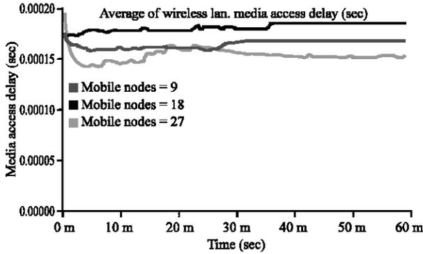
Fig. 8: Affect of number of nodes on media access delay
