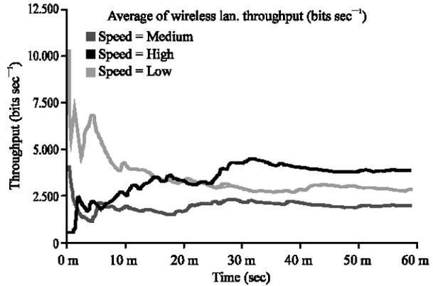
Fig. 7: Affect of speed on throughput
