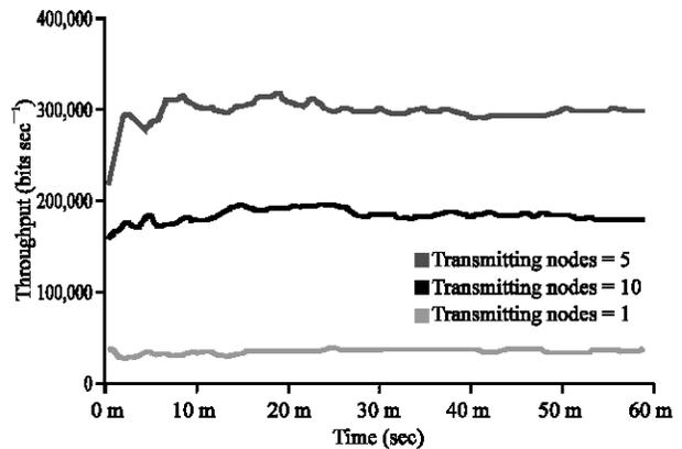
Fig. 11: Affect of number of transmitting nodes on throughput
