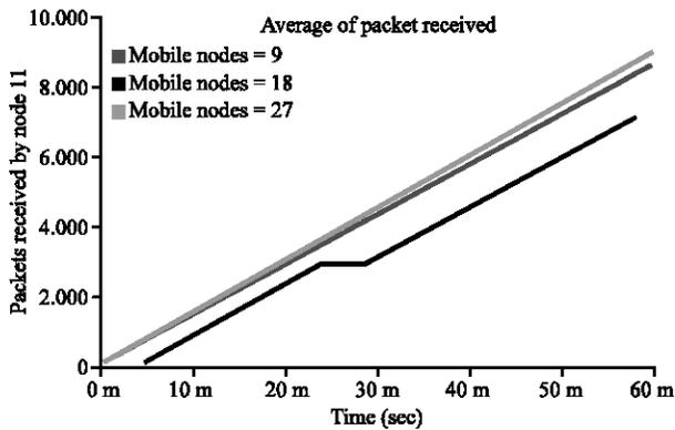
Fig. 9: Affect of number of nodes on packets reaching node 11
