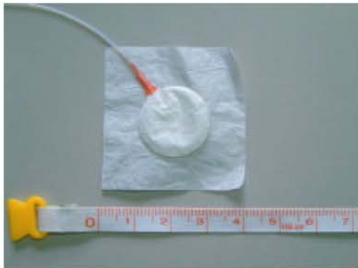
Fig. 2: AMI Ψ 20/2 m air-pack type pressure sensor
