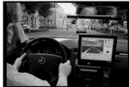
Fig 1: On-board implementation of the pedestrian detection system (Picture source: Gavila, 2000)
