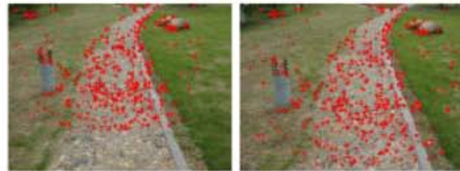
Fig. 9: Example of SURF matching results between 2 consecutive images by Shen and Liu (2007)
