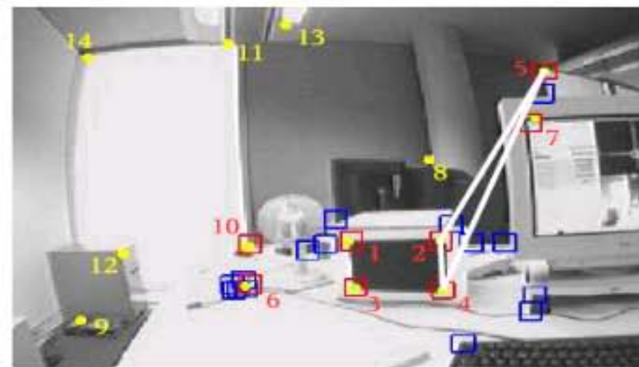
Fig. 4: Results of Williams et al. (2007) three point pose algorithm that finds up to four valid poses for the camera given the position in 3D
