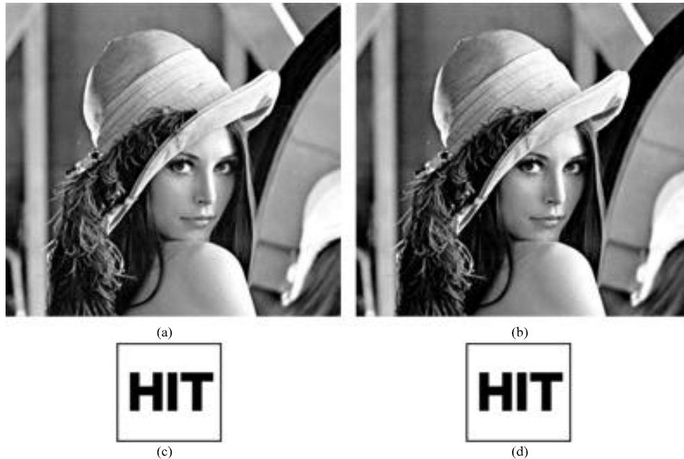
Fig. 2: The cover and watermarked images and the original and extracted watermarks without any attack, (a) Original cover image, (b) Watermarked image, (c) Original watermark and (d) Extracted watermark
