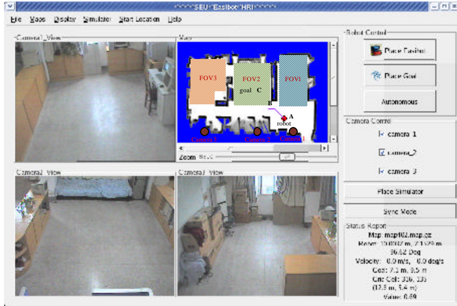
Fig. 8: The software interface including the experimental map and FOV of three cameras
