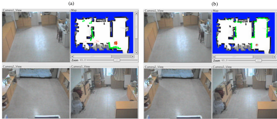
Fig. 10: The localization process using all information of three cameras. (a) The particles represent the robot's belief by integrating the negative information of three cameras and (b) Archived localization after 8 sec
