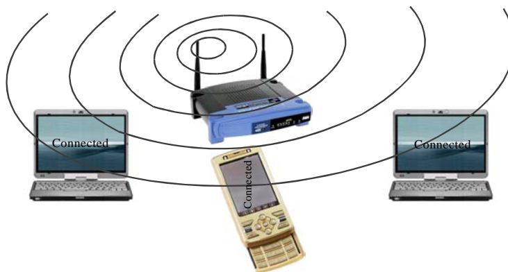
Fig. 1: The diagram illustrates how one wireless router can be used to connect several devices to the internet
