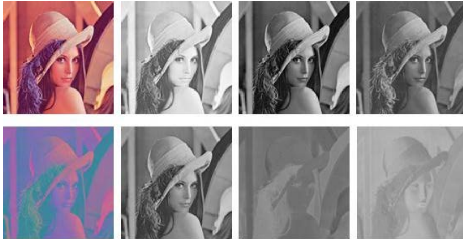
Fig. 1: Color channel decomposition of the 512×512 image Lena: the original image in the RGB space and the R, G and B channel planes (the top row, from left to right); the transformed image in the YCbCr space and the Y, Cb and Cr channel planes (the bottom row, from left to right)
