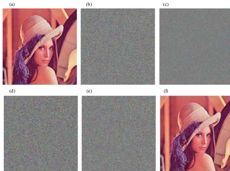
Fig. 3: Experimental results on the Lena image, (a) the original image, (b) the permuted image in the RGB color space, (c) the permuted image in the YCbCr color space, (d) the encrypted image with three times of iterations, (e) the decrypted image in the RGB color space before inverse permutation and (f) the decrypted image with PSNR = 100.23 dB
