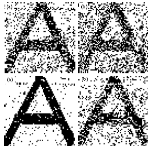
Fig. 7: Extracted watermark (a and b) Gaussian noise 0.1 and 0.3% and (c and d) sharpening and resizing, respectively
