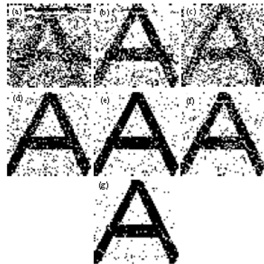
Fig. 6: Extracted watermark (a and b) JPEG compression with quality factor 85 and 90% and (c-e) salt and pepper noise (10, 3 and 1%) and (f and g) LPF and histogram equalization, respectively
