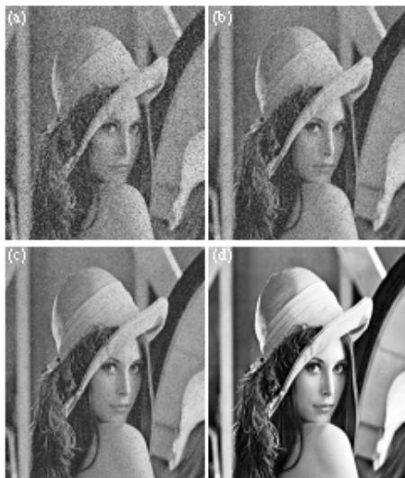
Fig. 5: (a-c) Distorted watermark image with salt and pepper noise (10, 3 and 1%) and (d) histogram equalization, respectively
