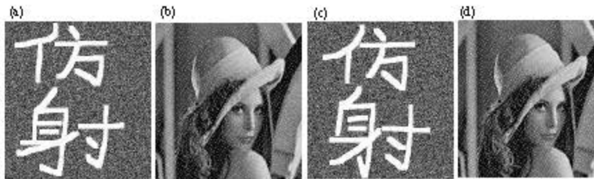
Fig. 6: The cutting effect and decrypting by uniform algorithm. (a) encrypting one time and cutting, (b) decrypting with a, (c) encrypting 64 times and cutting and (d) decrypting with c
