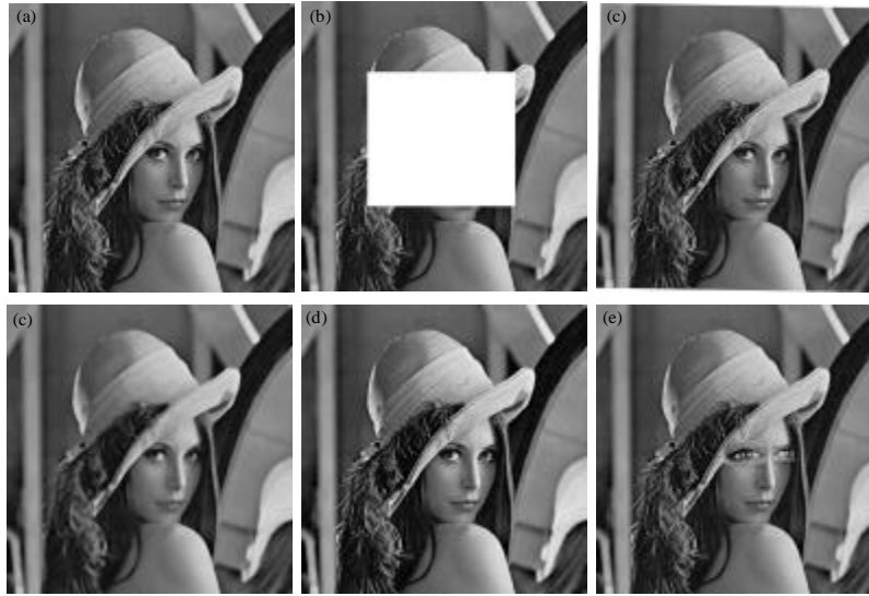
Fig. 5: The attacked Lena images. (a) JPEG compression with QF = 50, (b) cropping in the middle part of the image, (c) rotation by angle 1^\circ , (d) median filtering with the radius of 3 pixels, (e) contrast enhancement by 10% and (f) alteration of eyes
