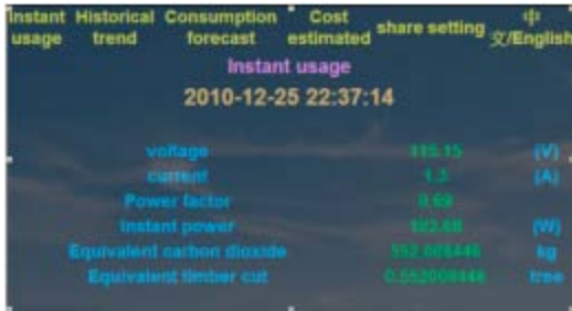
Fig. 4: Screen shot of instant power consumption
