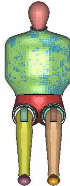
Fig. 2: Finite element model of SID (Side Impact Dummy)
