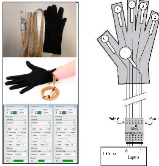
Fig. 5: I-CubeX glove sensors and multiple handle systems
