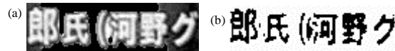
Fig. 8: (a) Modify background intensities of Fig. 5a and (b) proposed algorithm binarization result
