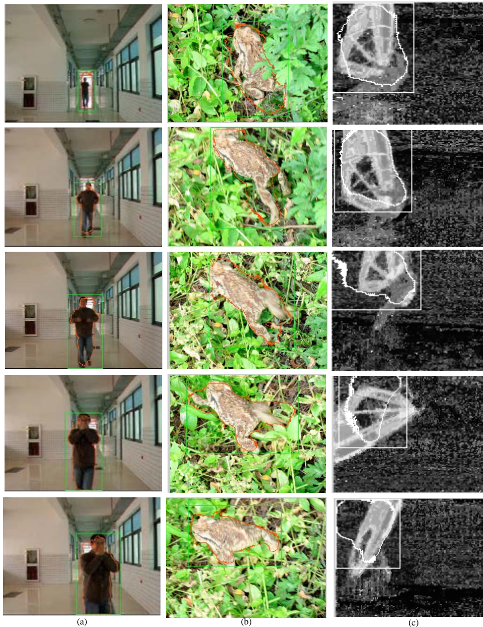
Fig. 2(a-c): Several different moving object segmentation results obtained by GMMLS: (a) a person towards a quivering camera in indoor scene, (b) a frog in dynamic grasses scene and (c) a surfer on dynamic water surface
