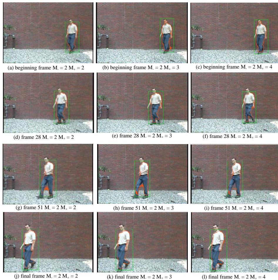
Fig. 1(a-l): A group of motion segmentation results on a moving person in front of a fixed camera obtained by GMMLS with different M (foreground) and M_+ (background)
