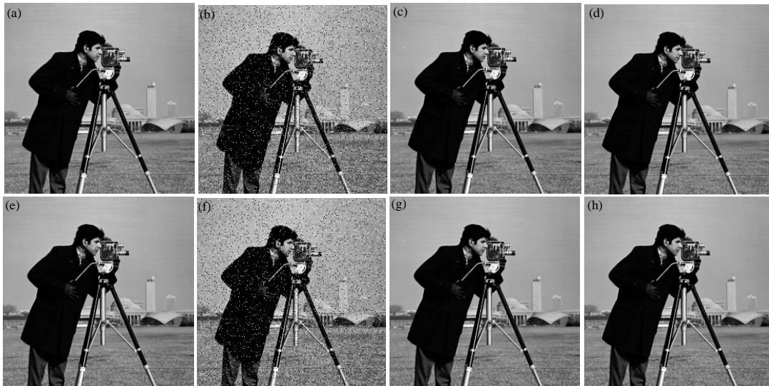
Fig. 6(a-h): Restoration performance comparison of different methods in filtering the image corrupted by random-valued impulsive noises at various noise ratios. (a-b) original image, (c) noised image ( p = 15\% ), (d) noised image ( p = 25\% ), (e-f) the restoration results of VSMF and (g-h) the restoration results of ARBMF
