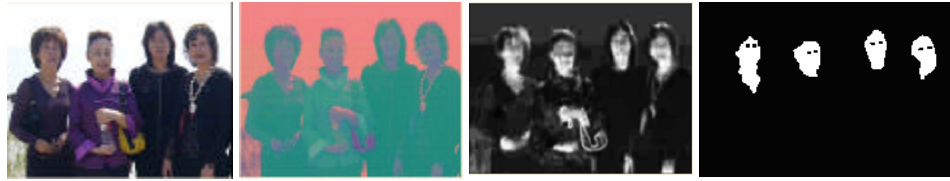
Fig. 4: Skin image segmentation process. From left to right: the original, the YCbCr color space, the skin probability, the segmented image
