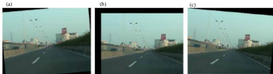
Fig. 8: The sample frames of the simulated In-Car videos of different categories. (a-c) are the frames of the videos of rotational only category, translational only category and compounded category, respectively
