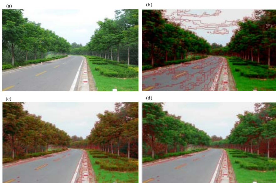
Fig. 2: Compare on structural road segmentation result. ((a) The primary image, (b) the edge extracted on H (Zhan and Jia, 2008; Shao-Qiu, 2009), (c) the edge on gray image (Zhang et al. , 2007) and (d) the edge extracted with this study method)
