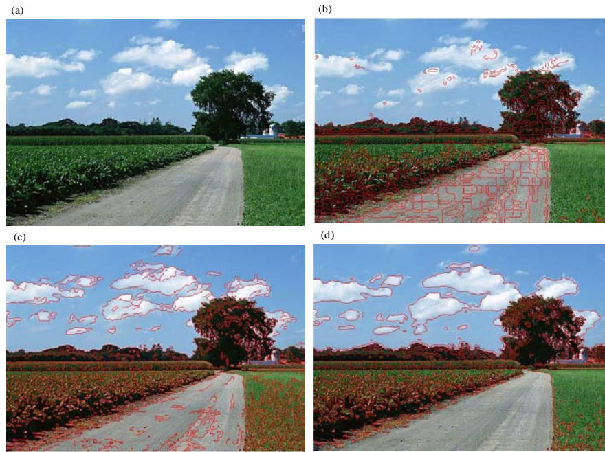
Fig. 3: Compare on un-structural road segmentation result. ((a) The primary image, (b) the edge extracted on H (Zhan and Jia, 2008; Shao-Qiu, 2009), (c) the edge on gray image (Zhang et al. , 2007) and (d) the edge extracted with this study method)
