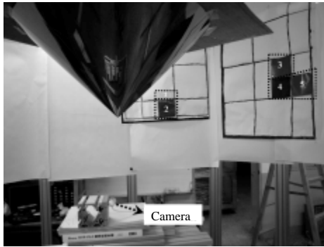
Fig. 7: Camera captures five images of color square via the conical mirror
