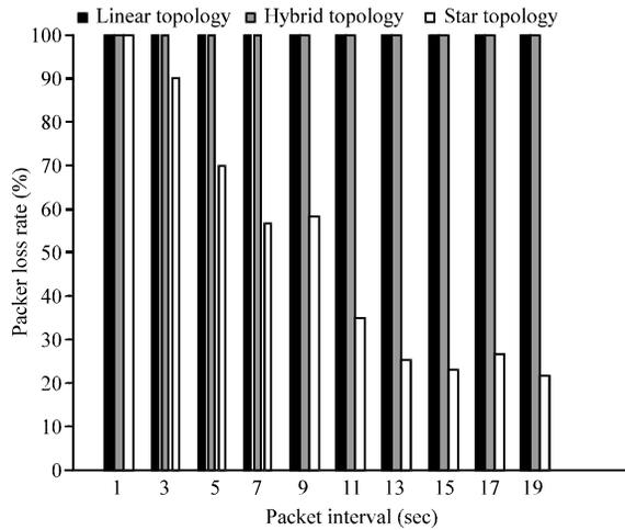
Fig. 8: Packet loss rate comparing (30% duty cycle)
