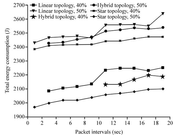
Fig. 7: Total energy consumption of networks based on three kinds of topologies
