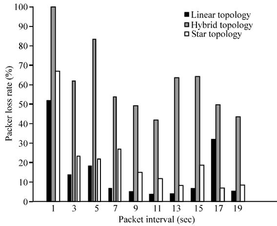
Fig. 10: Packet loss rate comparing (50% duty cycle)
