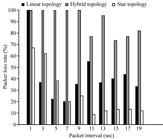
Fig. 9: Packet loss rate comparing (40% duty cycle)
