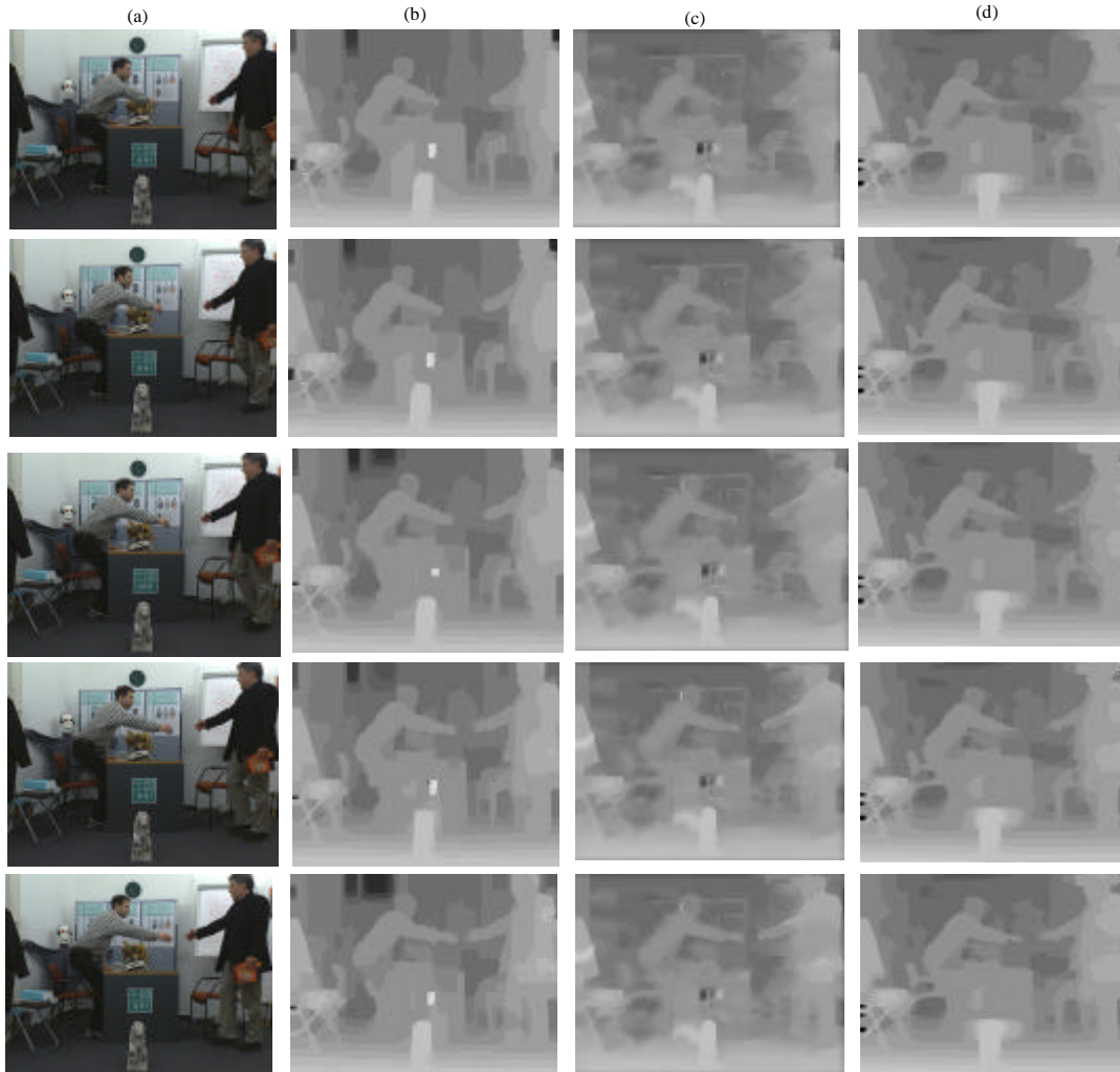
Fig. 4 (a-d): Disparity map results of different methods of frame 27 to 31 (from top to bottom) on the ‘book arrival’ sequence. (a) Source sequence; (b) Hierarchical BP method without temporal improvement; (c) adaptive window-based method with temporal smoothing filter and (d) Proposed method
