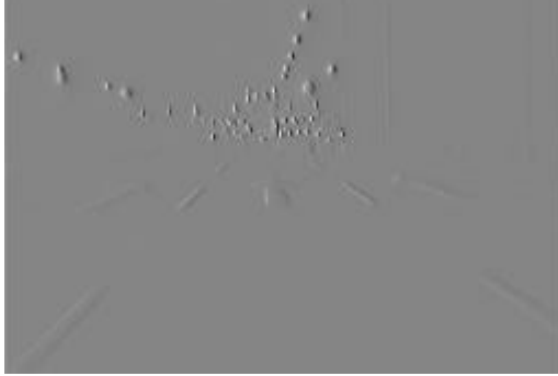
Fig. 4: Edge image by vertical Sobel operator
