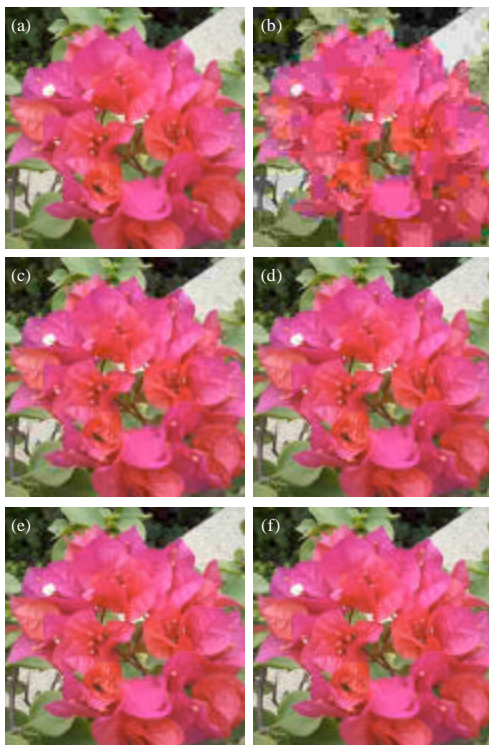
Fig. 10(a-f): Comparison chart of different layered compression images (a) Original image, (b) DC coefficient ( L_0 layer), (c) L_0+L_1 , (d) L_0+L_1+L_2 (e) L_0+L_1+L_2+L_3 and (f) L_0+L_1+L_2+L_3+L_4
