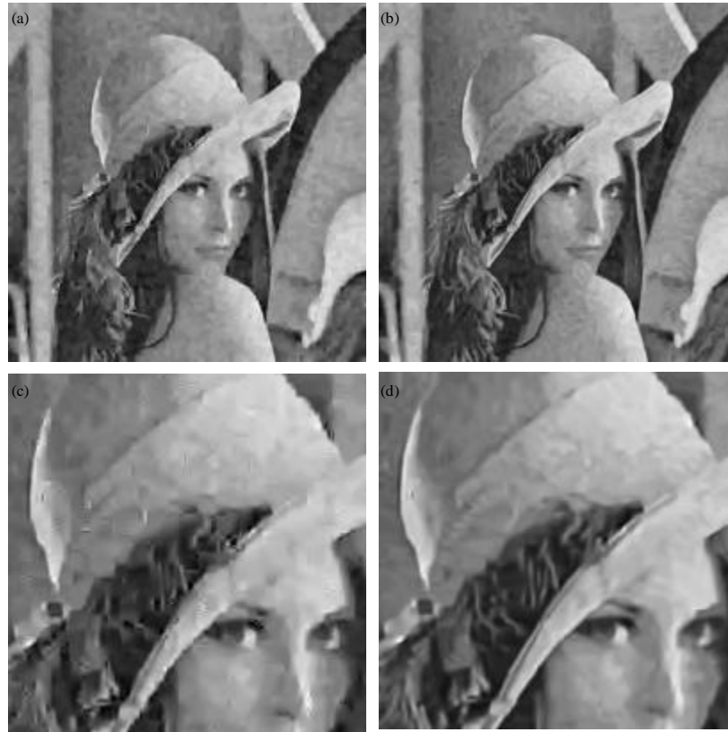
Fig. 6(a-d): Experimental results for image Lena512 ( \sigma = 60 ) (a) Result of BM3D, PSNR = 26.69 dB, SSIM = 180.62; (b) Result of our method, PSNR = 27.76dB, SSIM = 193.46; (c) Fragment of image (a); (d) Fragment of image b
