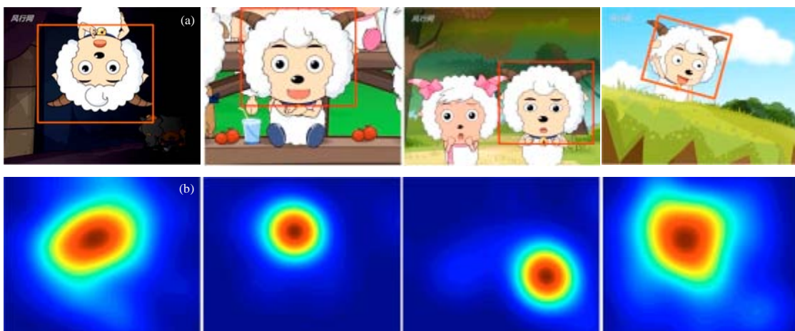
Fig. 7(a-b): Result of detection the cartoon character Xiyangyang (a) Original images with the red square marking the detection results and (b) Hough voting space of each image in (a)
