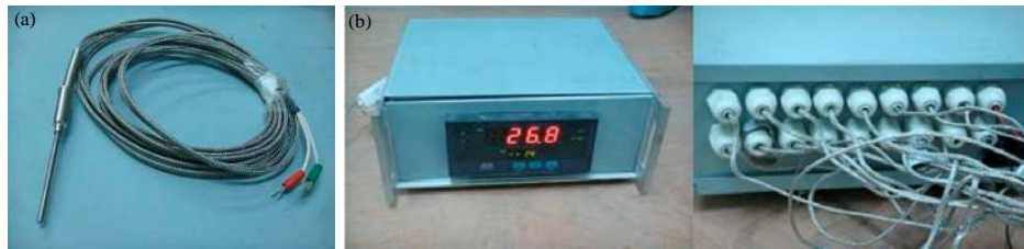
Fig. 1(a-b): Thermocouples and temperature patrol instruments used in the test, (a) Thermocouple and (b) Temperature patrol instrument
