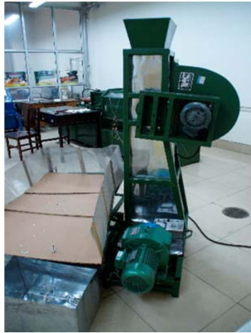
Fig. 6: The Winnowing and vibration sorting prototype
