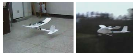
Fig. 6: Flight test at the hovering helicopter mode and fixed wing mode
