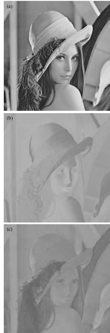
Fig. 3(a-c): \alpha\beta transform of sub-image (a) 1 component, (b) \alpha component and (c) \beta component
