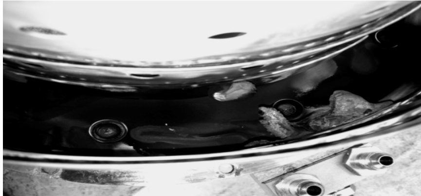
Fig. 8: Carbon deposition from fuel spray
